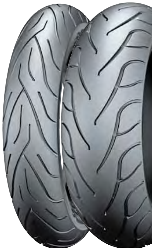
◀ Commander II 90-thread ply is 25% more dense than conventional plies
